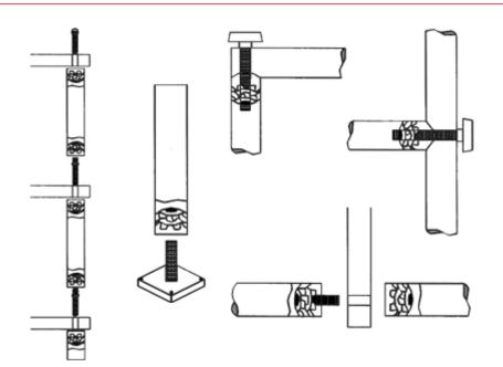
Inside Tube Diameter = 34,8-36,1Outer tube diameter =  $1 \frac{1}{2}$ " Thread = M6
